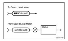
Fig. 8.26 Syntax for the HAndshake query message and sound level meter response
