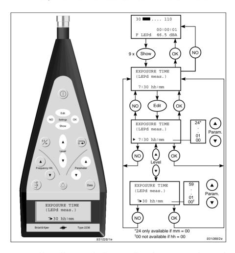
**Note:** Changing the Exposure Time does not reset the sound level meter. Therefore, you can investigate the effect of different Exposure Times on the  $L_{\rm EP,d}$  after a measurement.
