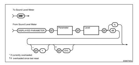
Fig. 8.15 Syntax for the DISp query message and sound level meter response
