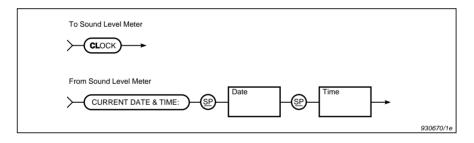
Fig. 8.11 Syntax for the CLock query message and sound level meter response
