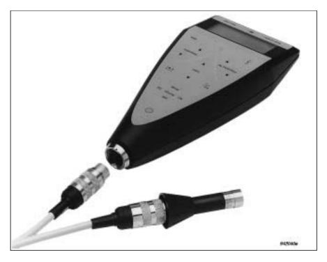
Fig. 3.2 Connecting a microphone extension cable to the sound level meter
