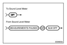
Fig. 8.27 Syntax for the OFf command
