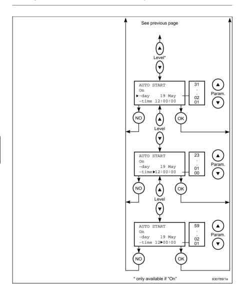
Auto Start only works if the sound level meter is switched off at the set time. Then, at this time, the sound level meter will switch on, reset and, after a pause of 5 seconds, start measuring with the set-up it had when it was switched off.
