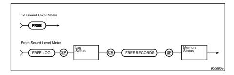
Fig. 8.22 Syntax for the FREE query message and sound level meter response
