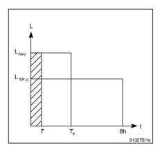
Fig. 8.2  $L_{EP.d}$  compared to  $L_{Aeq}$
