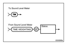
Fig. 8.40 Syntax for the TW query message and sound level meter response
