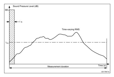
Fig. 8.1 SEL compared to weighted  $L_{eq}$
