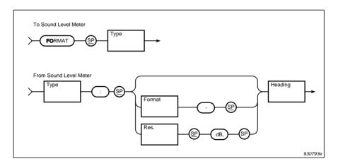
Fig. 8.21 Syntax for the FOrmat query message and sound level meter response
