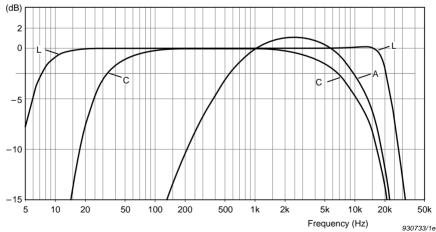
Fig. 6.1 Nominal frequency weighting characteristics
