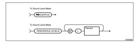
Fig. 8.30 Syntax for the PErcentile query message and sound level meter response
