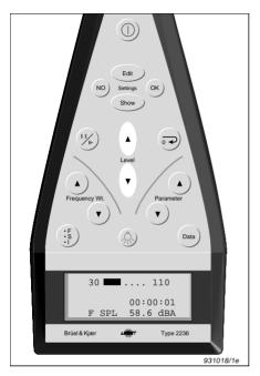
To move the measurement range by 10 dB, press **Level**  $\langle \blacktriangle \rangle$  or  $\langle \blacktriangledown \rangle$ , respectively.\*
