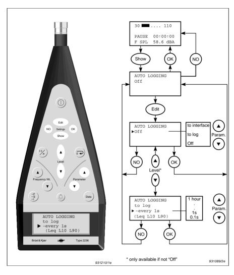
If you change the range or the frequency or time weighting while the sound level meter is set to log results in the sound level meter's memory, the sound level meter stops logging and auto logging is set to Off. This is because the measurement set-up information in the log would no longer be relevant for further logged results.
