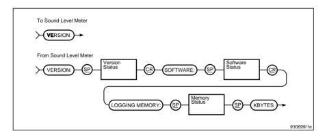
Fig. 8.41 Syntax for the VErsion query message and sound level meter response
