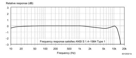
Fig. 6.6 Typical diffuse-field response of Microphone Type 4188 with random incidence corrector
