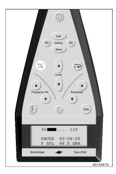
The Pause mode of the sound level meter allows you to store results in its memory or transfer results across the interface to a printer or computer.
