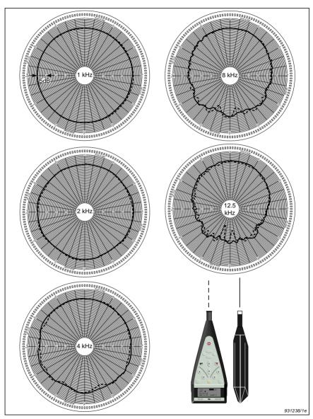
Fig. 6.7 Directional characteristics of the complete instrument at 1, 2, 4, 8, 12.5 kHz
