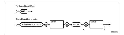
Fig. 8.7 Syntax for the BATt query message and sound level meter response
