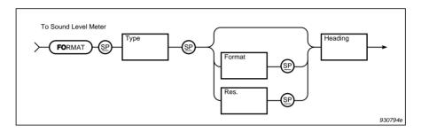
Fig. 8.20 Syntax for the FOrmat command
