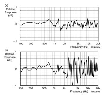
Fig. 6.8 (a) Effect of the sound level meter's casing on its frequency response (for reference) compared to (b) the effect of Tripod UA 0801 on the sound level meter's frequency response
