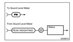
Fig. 8.33 Syntax for the PW query message and sound level meter response
