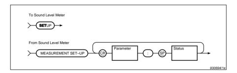
Fig. 8.37 Syntax for the SETup query message and sound level meter response
