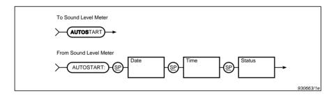
Fig. 8.6 Syntax for the AUTOStart query message and sound level meter response
