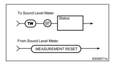
Fig. 8.39 Syntax for the TW command
