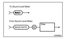
Fig. 8.9 Syntax for the BAUd query message and sound level meter response
