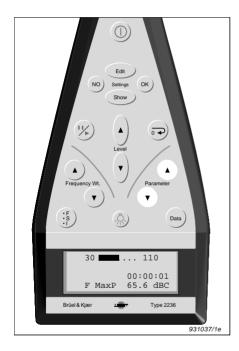
To step forwards and backwards through the available parameters, press **Parameter**  $\langle \blacktriangle \rangle$  or  $\langle \blacktriangledown \rangle$ , respectively.
