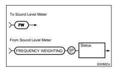
Fig. 8.24 Syntax for the FW query message and sound level meter response
