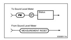
Fig. 8.23 Syntax for the FW command
