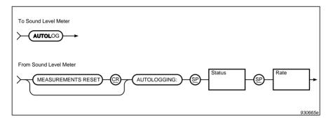
Fig. 8.4 Syntax for the AUTOLog query message and sound level meter response
