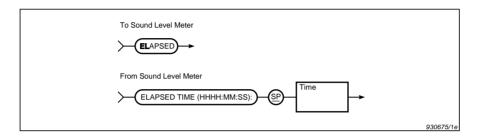
Fig. 8.16 Syntax for the ELapsed query message and sound level meter response
