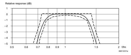
Fig. 6.3  $^{1}$ / $_{1}$ -octave filter characteristics as a function of frequency, f, against centre frequency, f<sub>m</sub> (detail of Fig. 6.2). IEC tolerances are shown as dashed lines
