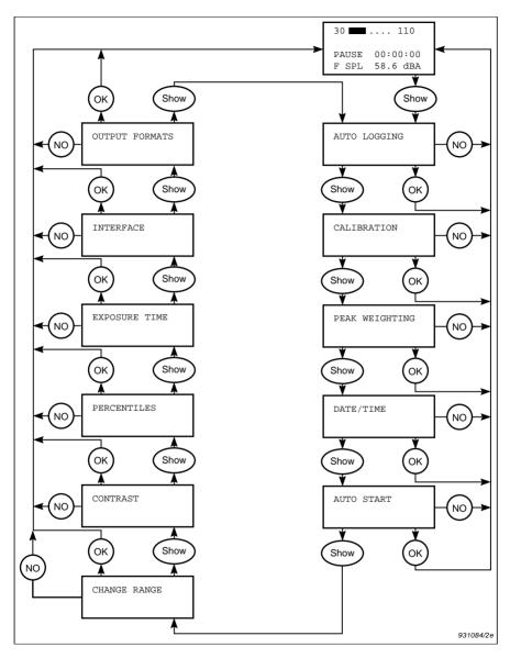
Fig. 1.2 An overview of the sound level meter's Settings
