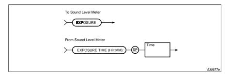
Fig. 8.19 Syntax for the EXPosure query message and sound level meter response
